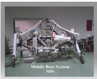
The foundation of the MSS, this system will be employed as a working Platform and storage area
